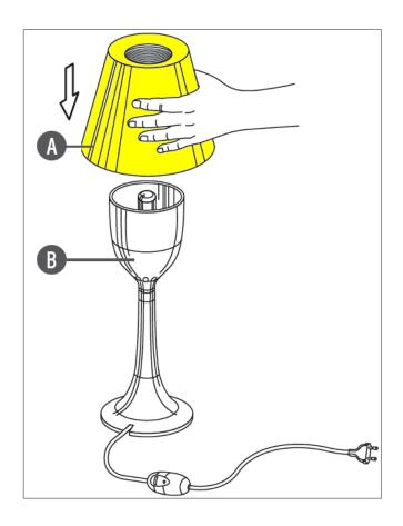
Lock the external diffuser (A) to the inner diffuser (B) by forcing (pushing) it, until it clicks-on.
