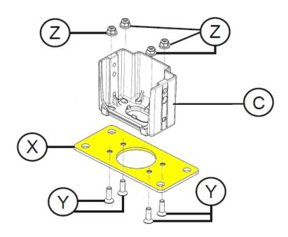
ONLY FOR EARTH FIXING. If perhaps the earth surface is not stable, it is necessary to level the surface through the stability plate or bracket. Install the stability plate (X) by utilizing the armed expansion plugs and fix the plate with the relative screws (Y) and nuts (Z).
