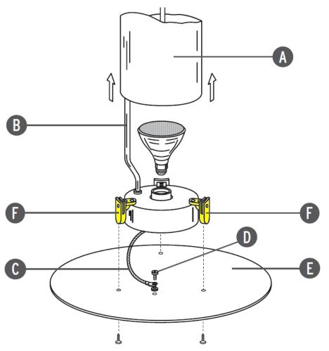
Remove the diffuser (A) from the metal stem (B). Unfasten the "PAR" bulb from the lower lampholder. Remove the base (E) from the supports (F) by unfastening the three self-threading screws.
