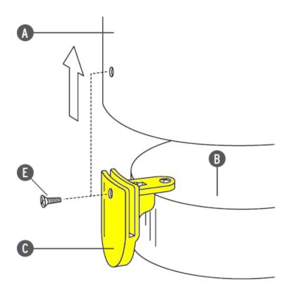
Unfasten the three screws (E) from the support (C) and then lift-up the diffuser (A).
