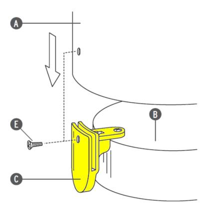
Insert the diffuser (A) into the metal structure (B) and through the openings in the supports (C). Utilize the tip of a screwdriver to help your self if necessary to align the holes in the diffuser to correspond with those present on the support. Assemble the diffuser (A) by fastening screws (E).
