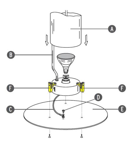
Connect the earth cable (C) to the base by fastening the screw (D), ensuring to insert the cable between the screw and the notched washer; Assemble the base (E) to the supports (F) by fastening the three self-threading screws. Screw the "PAR" bulb into the lower bulbholder. Slide the diffuser (A) through the metal stem (B).
